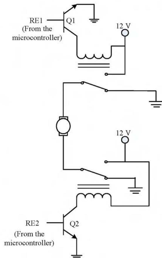
Fig. 3 The Circuit Diagram of Motor Controller Circuit
