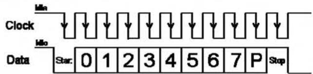
Fig. 4 The Waveform Diagram of One Byte Transmission from the Keyboard
