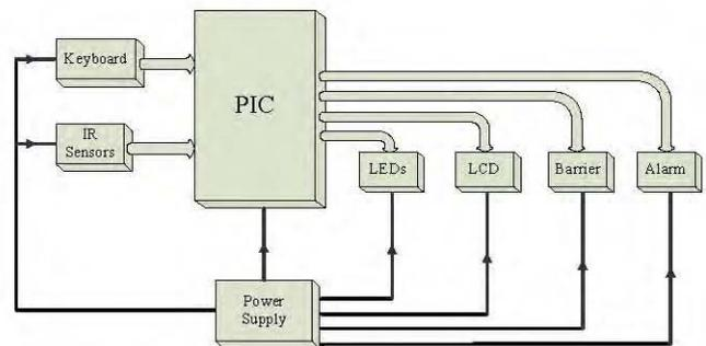
Fig. 1 Block Diagram of Car Parking Control System
