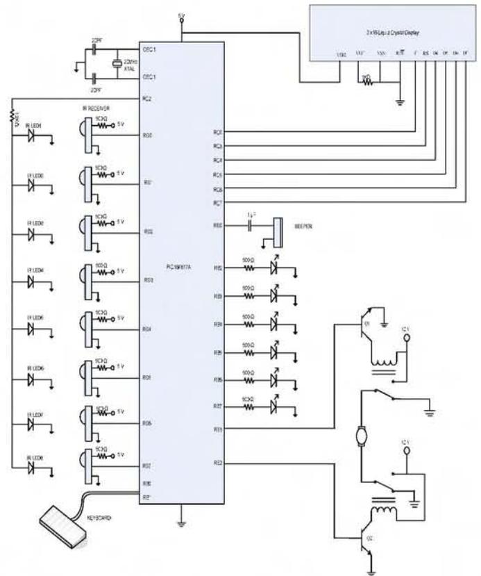
Fig. 5 Overall Circuit Diagram of the System
